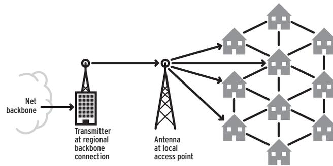
**FIGURE 13 – WIRELESS LAST MILE:** In one wireless last-mile scenario, a transmitter tower connected to the Internet transmits in a point-to-point connection to a community access point, which makes point-to-multipoint or mesh network connections to households.
