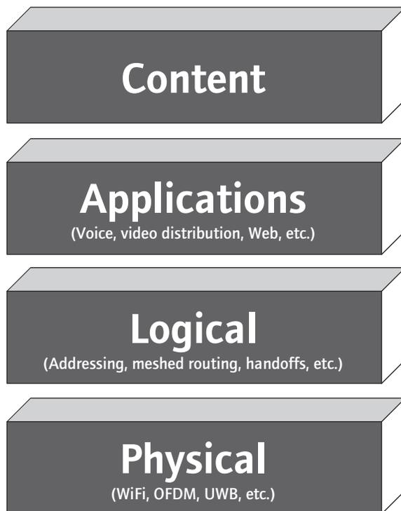
**FIGURE 4 – LAYERS:** In the digital era, wireless signals consist of a stream of interchangeable digital bits. Engineers use a layered framework to provide order and optimize and manage transmissions.
