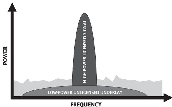
**FIGURE 10 – UNDERLAY SHARING:** In underlay sharing, low-power, unlicensed devices share frequencies and avoid interference by operating beneath the noise threshold of high-power devices in the band.
