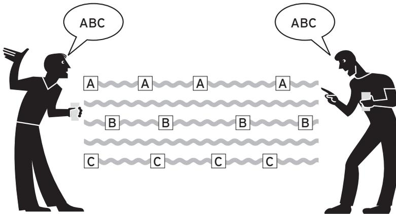
**FIGURE 7 – SPREAD SPECTRUM:** In spread-spectrum communications, low-power radio transmitters divide their signals into coded packets across a range of frequencies and receivers reconstruct the message.
