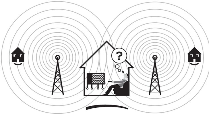
**FIGURE 1 – NOTIONS OF INTERFERENCE:** When two or more signals share the same space at the same time, some receivers have difficulty distinguishing them and interference can result.
