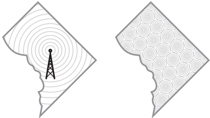
**FIGURE 3 – COMPARING BROADCAST VS. CELLULAR ARCHITECTURE:** The broadcast architecture (left) services more users over a larger area with one signal, while the cellular architecture (right) lets more users receive and send distinct transmissions.
